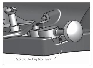
Use a 1/16" hex key to loosen the set screw. Once the slow adjuster has been installed, tighten the set screw back in only as far as the adjuster cannot be removed, but can still pivot freely.
